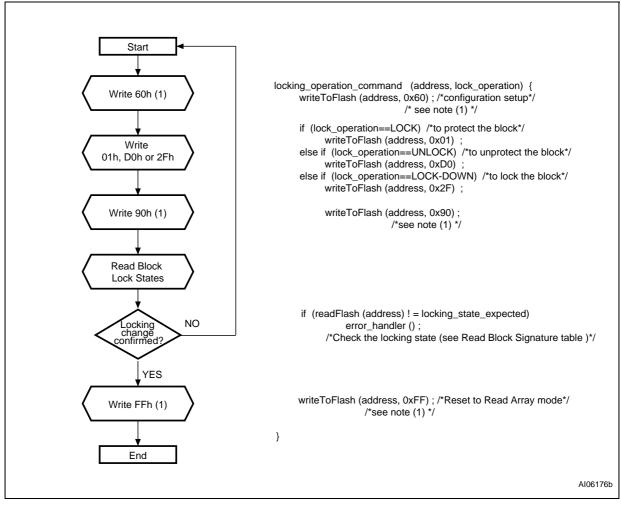
Figure 26. Locking operations flowchart and pseudocode
