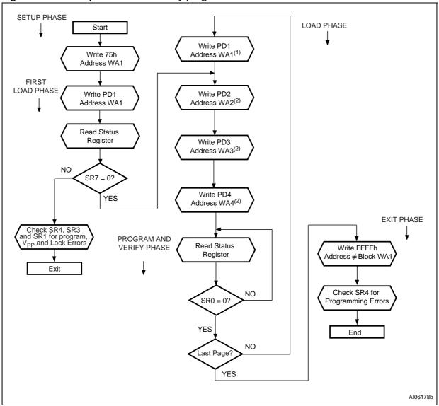
Figure 29. Quadruple enhanced factory program flowchart
